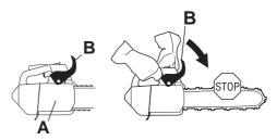
This movement activates a spring-loaded mechanism that tightens the brake band (C) around the engine drive system (D) (clutch drum).
